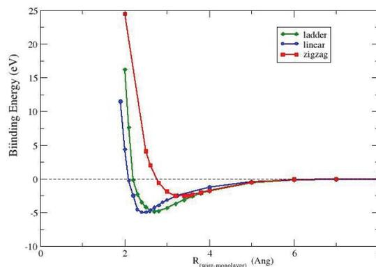
**FIGURE 2.** Binding Energy vs wire-monolayer separation ( $R_{\text{wire-monolayer}}$ ) curve for the assembled system.
