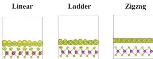
**FIGURE 4.** A side view of the valence band charge density of assembled systems with isosurface value  $0.003 \text{ e}/\text{\AA}^3$
