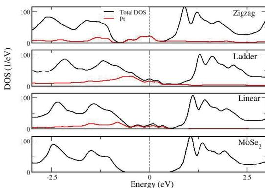
**FIGURE 3.** Density of States for Pristine and assembled system of MoSe<sub>2</sub>.
