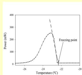
interception of a line fit to the leading edge of the peak with the baseline. The latent heat is the area under the curve when plotted as power vs. time. The result of a temperature calibration against the melting point of ice Ih is shown in the histogram to the left.
